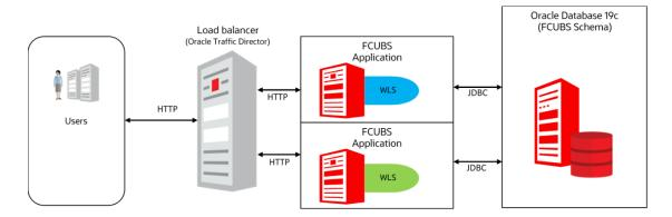
The Blue-Green deployment process uses two identical environments-Blue and Green. Only one environment is active at a time, serving all the traffic with the load balancer and the other environment is in the standby mode.
